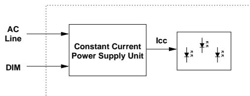
Fig. 1. Standard LED lamp
