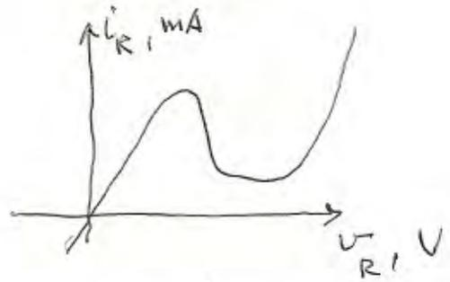
$$i_R = 17.7 V_R - 103.79 V_R^2 + 229.62 V_R^3 - 226.31 V_R^4 + 83.72 V_R^5 \text{ mA}$$
