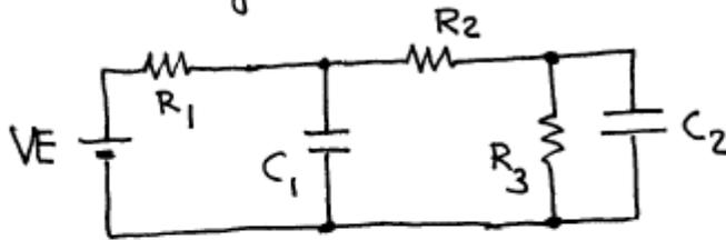
$$\begin{aligned} V_E &= 10 \text{ V} \\ R_1 &= 2 \text{ k}\Omega \\ R_2 &= R_3 = 5 \text{ k}\Omega \\ C_1 &= 10 \text{ nF}, C_2 = 10 \text{ nF} \end{aligned}$$
